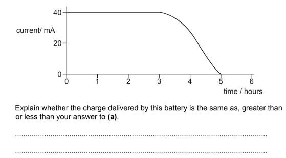
(b) Below is the graph of current against time for a different battery.
